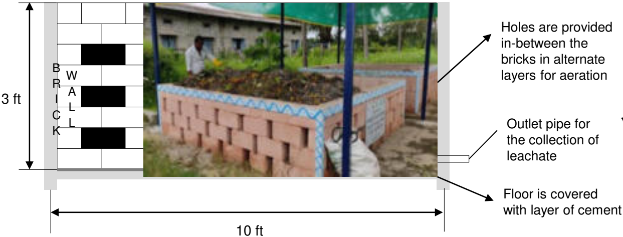
Side View of the tank
