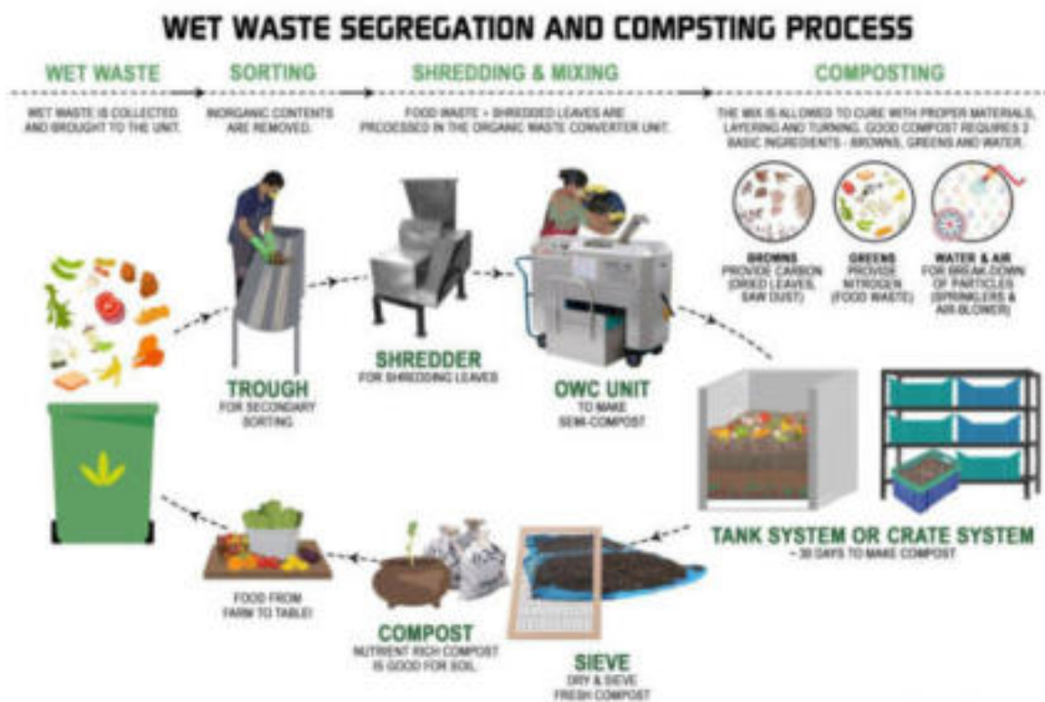
Figure 43: Wet Waste Segregation and Composting Process
