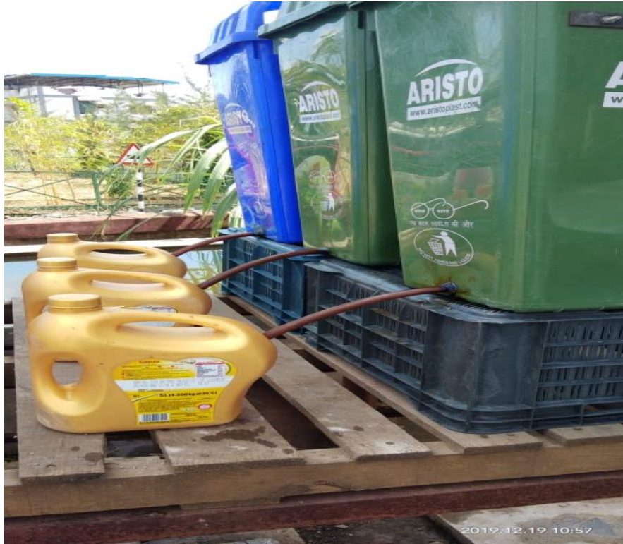
Ward No-23 Organic waste liquid composting
